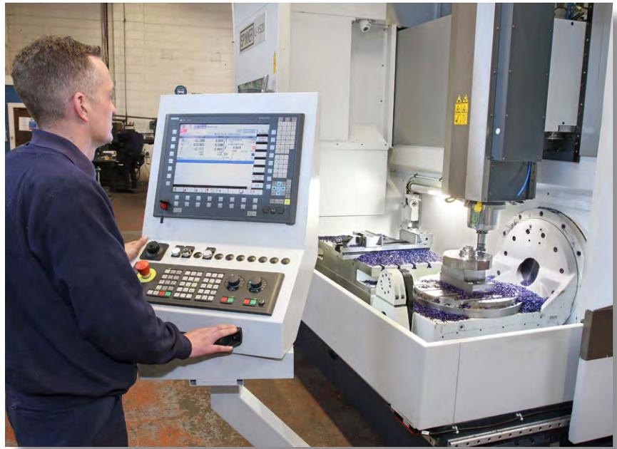
"There are a number of trunnion-type, five-axis machines on the market, but unusually on the Spinner the axis of rotation is from front to back. It gives added versatility by allowing the fixed table to be positioned adjacent to it in the X-axis, enabling the machining of long components that straddle both tables."
